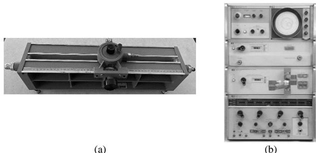
Fig. 9. Lab equipment. (a) Slotted transmission line. (b) HP 8410 vector network analyzer.
