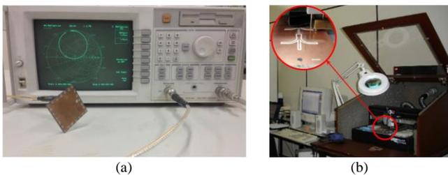
Fig. 12. Lab equipment. (a) VNA HP-8714. (b) T-Tech milling machine.
