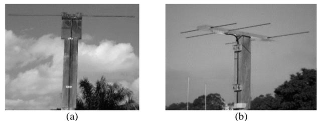
Fig. 7. Antennas used in CEM-20 laboratory classes. (a) electric dipole. (b) Yagi-Uda antenna.
