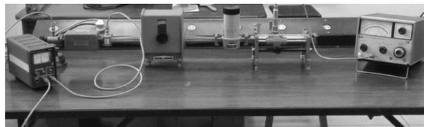
Fig. 10. Experimental setup with a slotted waveguide at the X band.
