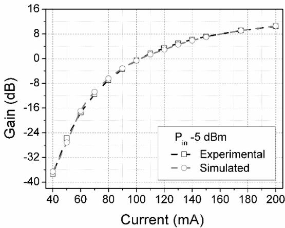
Fig. 4: Gain curve vs. bias current for the calibrated model and the experimental results for  $P_{in}$  (a) -5 dBm
