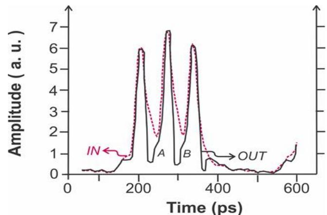
Fig. 6: Photo-detected signals for a 12 GHz microwave carrier after the SOA (red dotted line) and after 18 km of fiber propagation (continuous line).
