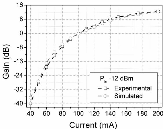
Fig. 5: Gain curve vs. bias current for the calibrated model and the experimental results for  $P_{in} = -12$  dBm
