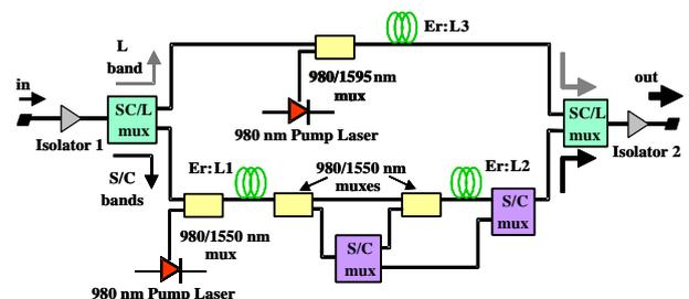
Fig. 1. Schematic diagram for the triple-band EDFA.
