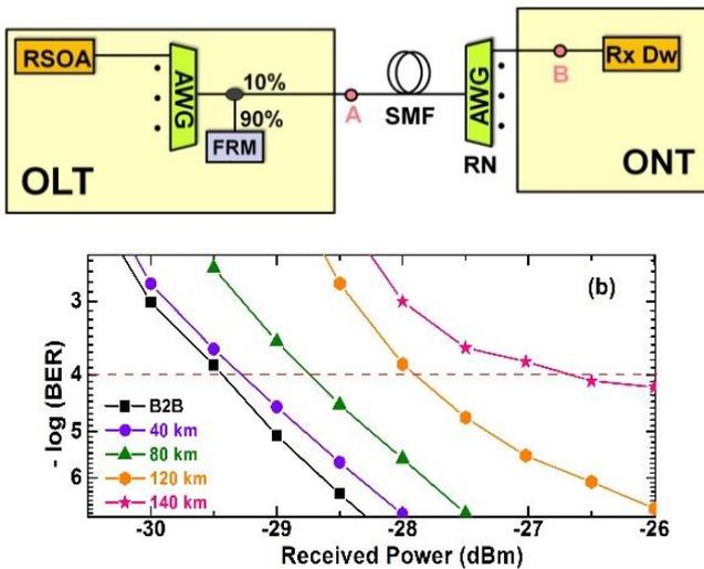
**Fig. 8: Top (a):** Self-seeding architecture where FRM is the Faraday rotator mirror, the reflective element used to avoid instabilities caused by polarization fluctuations. **Bottom (b)** BER optical transmission measurements up to 140 km [44].
