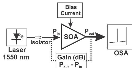
Fig. 3. Block diagram for the experimental setup.
