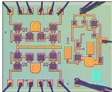
**Fig. 7:** Photo of the electronic channel selector circuit, part of an optoelectronic receiver for WDM-PON [40]. To the left, four microwave switches (3 FETs each, in a  $\pi$ -shaped connection) select the detected wavelength to be amplified by the transimpedance amplifier (right side).
