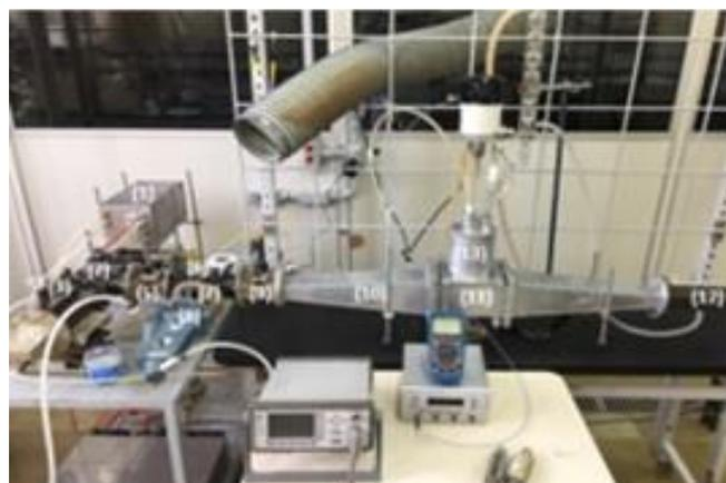
Fig. 3. Thermo-controlled reactor in a pyramidal cavity.
