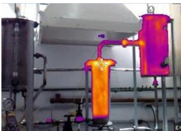
Fig. 2. Thermography of distillation column reboiler pilot in operation.
