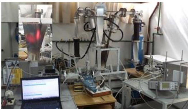
Fig. 6. Furnace for self-reducing iron ore pellets. The inset shows the outside surface of the reactor in operation.
