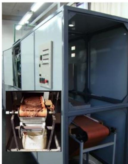
Fig. 1. Continuous microwave belt oven. Inset shows the dried iron ore at the output.
