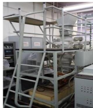
Fig. 5. Pilot for microwave-assisted rice parboiling.
