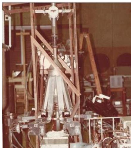
Fig. 4. Microwave assisted cassava saccharification pilot.
